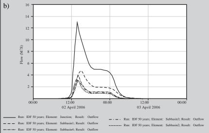
Figure 6. Hydrographs for each sub-basin and for the junction of the four sub-basins for a 24-hour storm event. a) for a 10 years return period; b) for a 50 years return period.
