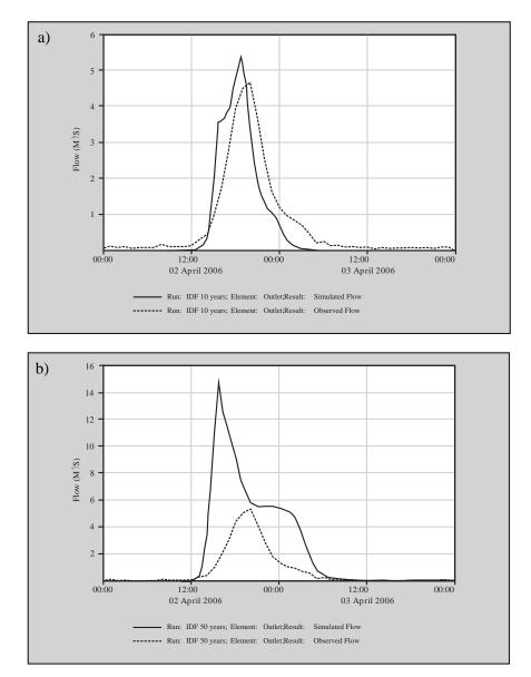
Figure 7. Flow comparison graph of the simulated and observed outlet flow for the Wadi Madoneh basin with return periods of (a) 10 years and (b) 50 years. Precipitation data from the Intensity-Duration-Frequency curve at Zarqa rainfall station.
