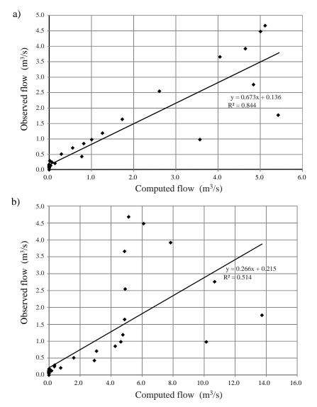
Figure 8. Flow comparison between observed and simulated flow using a (a) 10 years return period and (b) 50 years return period.
