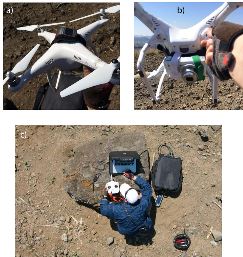
Figure 4. Set-up used in this study with a Phantom-2 quadcopter (diagonal length of 59 cm including propellers): (a) a portable GPS (Garmin Forerunner 305) attached on the top of the quadcopter in order to record flight data, (b) a Canon S110 placed on the bottom of the quadcopter pointing downward, and (c) DJI's ground station software was run on a portable computer in order to program all required flights—picture taken by the quadcopter during take-off.
