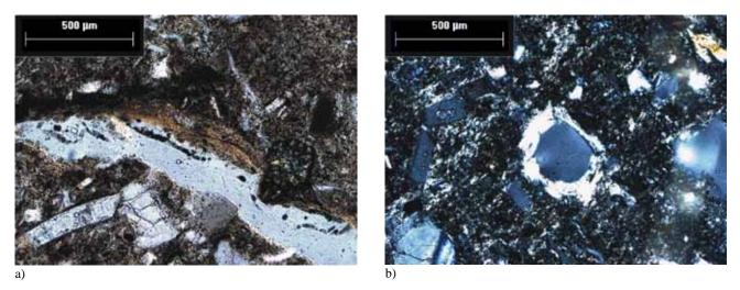
Figure 4. Micromorphological features of paleosol San Lorenzo. a) A dusty clay coating in a cavity of 2B horizon; b) neoformed carbonate of 3Bt horizon.
